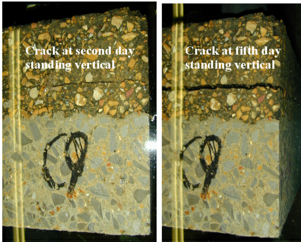
Figure 6.34. Delamination between asphalt layers on F&T specimen C9 at 64 cycles.
