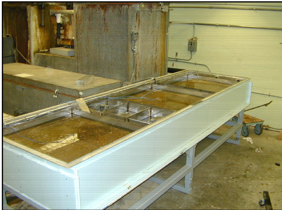
Figure 5.2. New F&T exposure tank (with three large and three small UTW samples).
