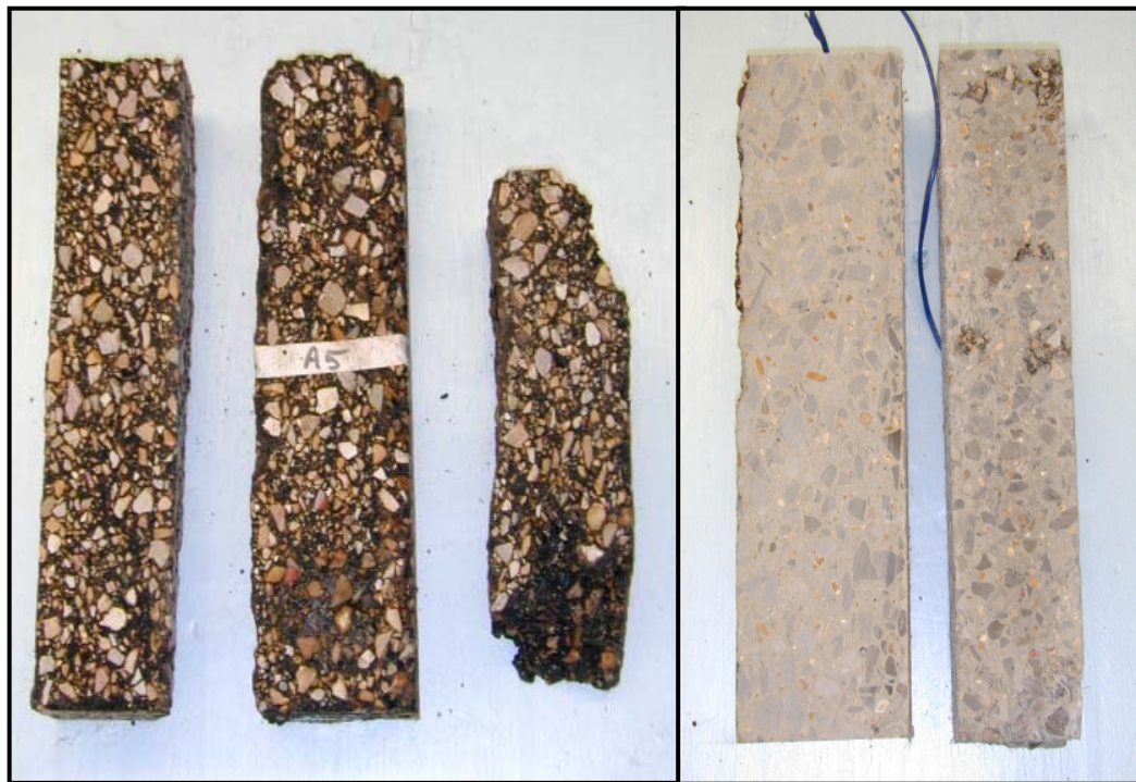
Figure 6.5. AC and PCC prisms were deteriorated using F&T exposures.
