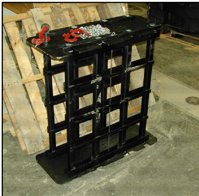
Figure 5.11. Frame used to handle specimen during transport in the laboratory.
