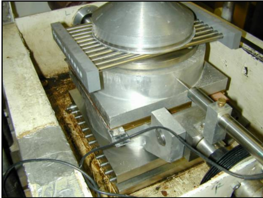
Figure 6.3. Shear rig for testing PCC/AC bond strength.
