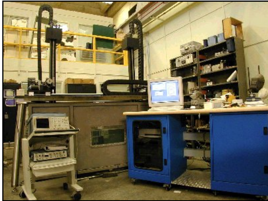
Figure 6.9. USUMS for imaging anomalies in large PCC specimens.
