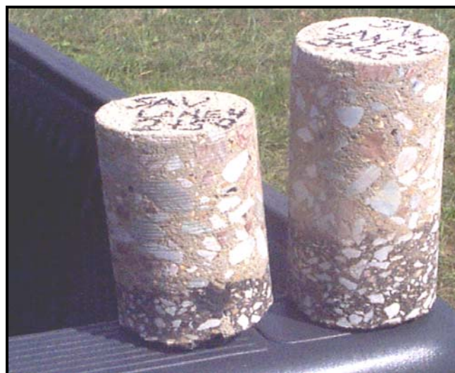
Figure 2.6. Cores extracted at SNH during construction indicated a good bond.
