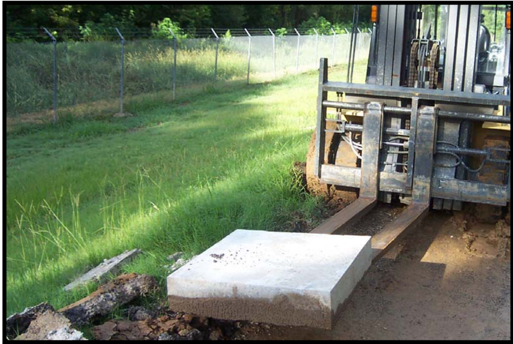
Figure 4.16. A forklift was used to remove large 34 inch by 34 inch samples.
