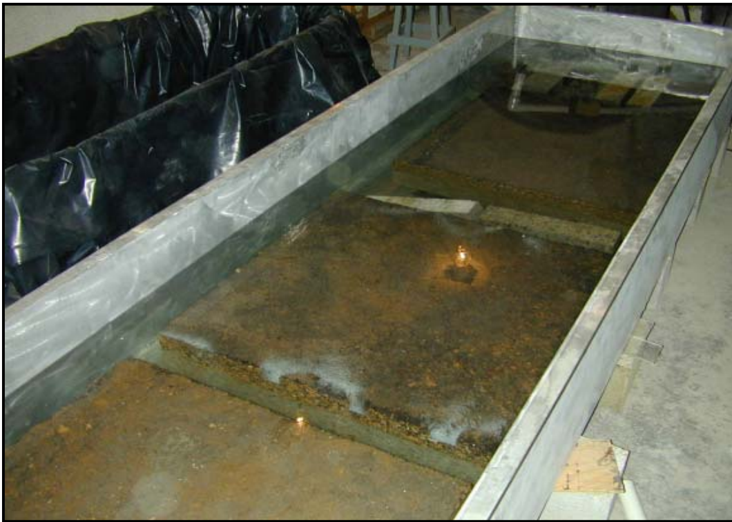
Figure 5.8. UTW specimens undergoing W&D exposure in the W&D tank.
