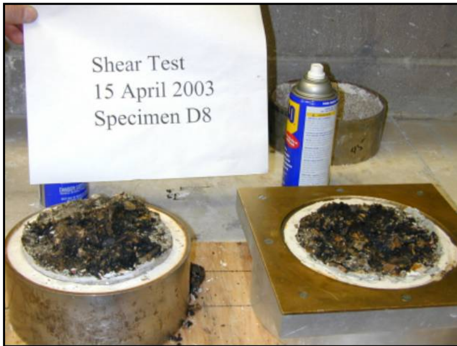
Figure 6.4. Shear test on PCC/AC bond.
