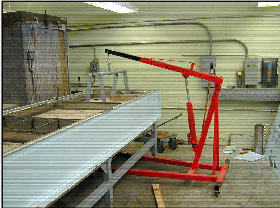
Figure 5.10. A 2-ton capacity crane was used to handle specimens in exposure stations.
