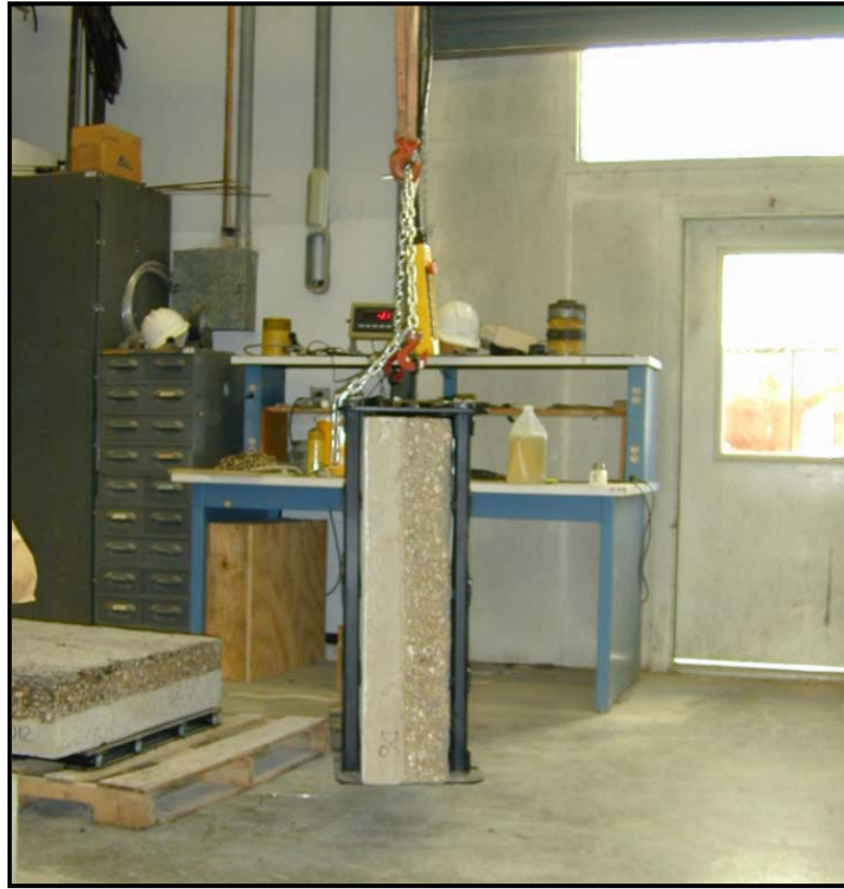
Figure 6.7. Winch for lowering and removing UTW specimen into scanning tank.
